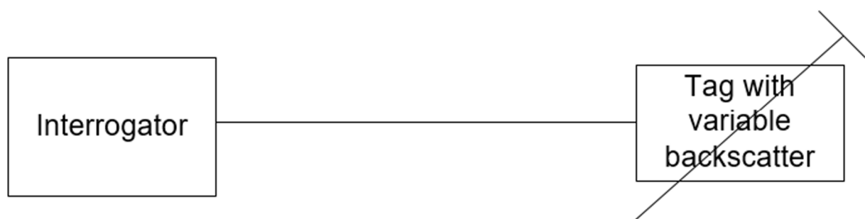
Figure 15b: Conducted test set up for receiver sensitivity with (emulated) tag with variable backscatter
